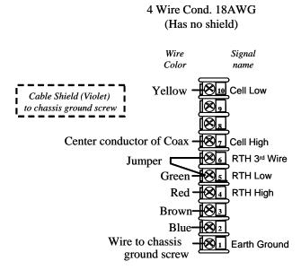
Figure 7-15 Terminal Designations for Conductivity Cells with Quick Disconnect
